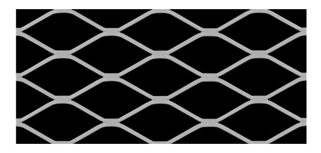
LW Aperture: 43.43mm Strand Width: 2.31mm SW Aperture: 18.03mm Thickness: 1.14mm Weight: 1.85 kg / m2 Open Area: 80%
